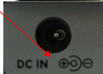
2 – Connect the power supply to Genius and to the electric current.
