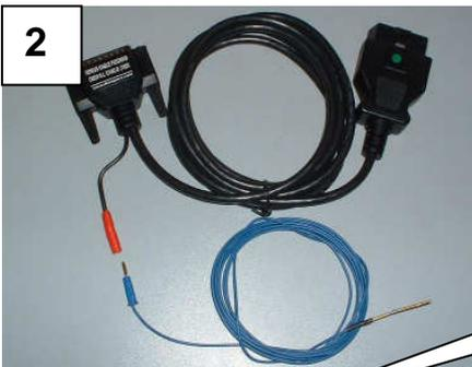
For this wiring you could find an OBDII socket or a typical BMW load connector
