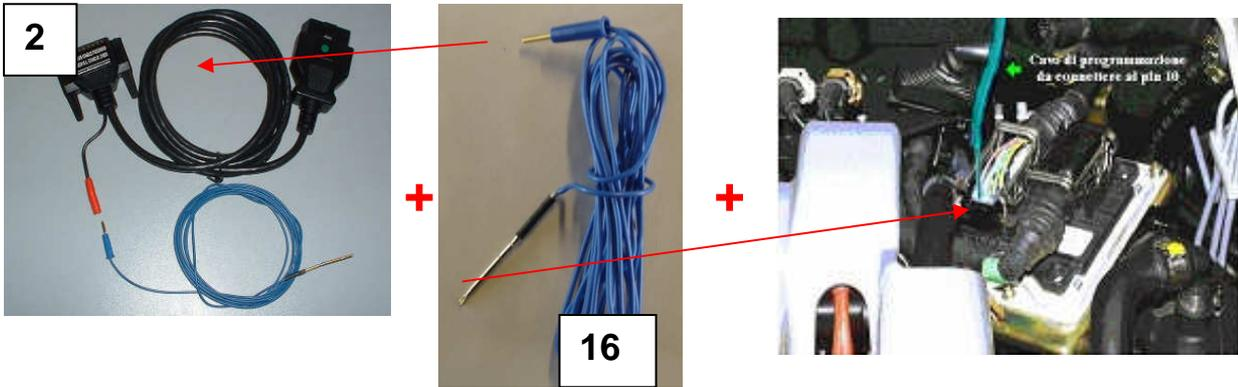
**CAUTION:** We must put one endpoint of the blue wire in the OBDII blue connector, the other one must be connected to the Pin 10 of the ECU.
