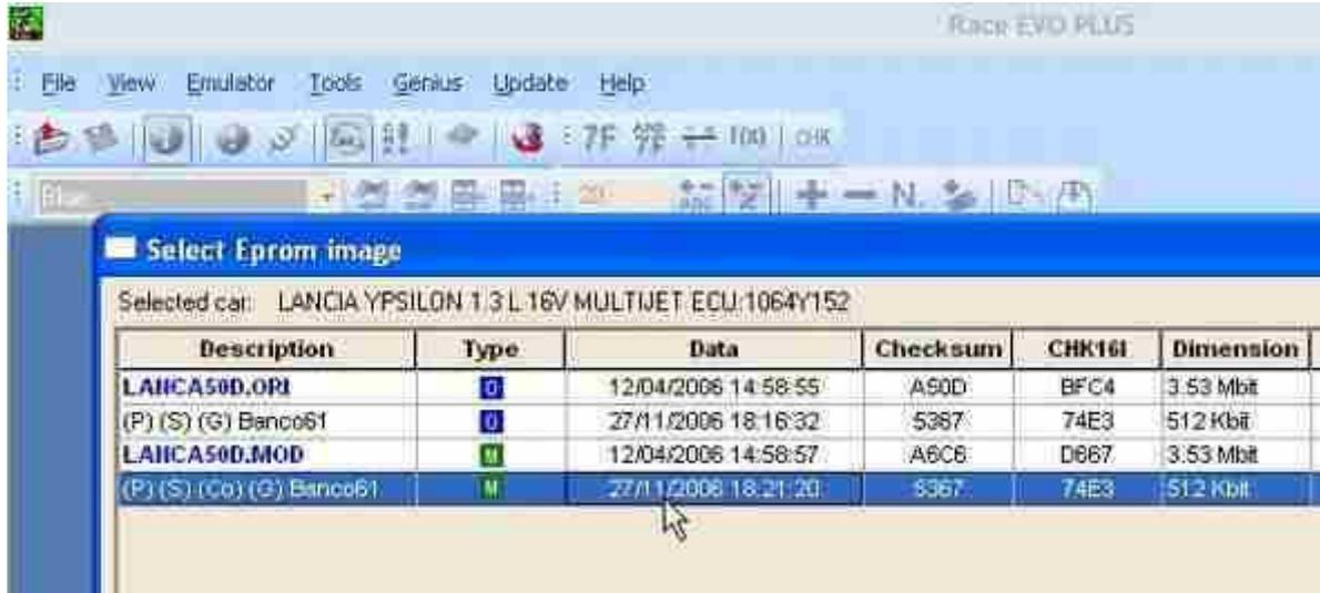
From the Genius button select **Write image to Genius**, be sure that the file **.MOD** is saved with name inside the folder "Write".
