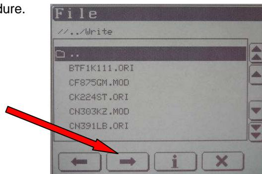
After selecting the file to write follow the procedure, in some cases Genius will ask to switch on and off the dash-board, it depends on the vehicle.
