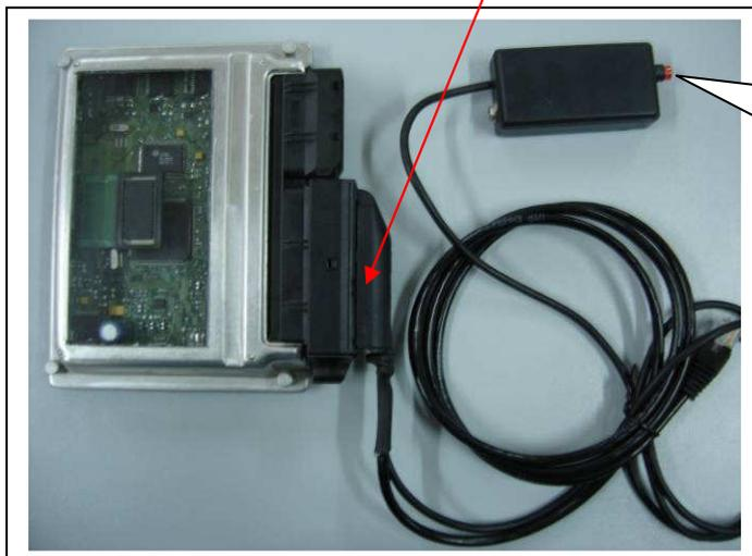
When the software RaceEVO shows you the message *Switch ON the dashboard* you must switch the red button , than when the system ask you to *switch OFF the dashboard* you must switch another time the red button.
