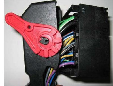
2 – In the connector look for the **PIN 43** that allows the communication with the ECU.
