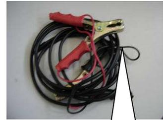
If you want you can obtain supply from +12V battery using the battery connectors
