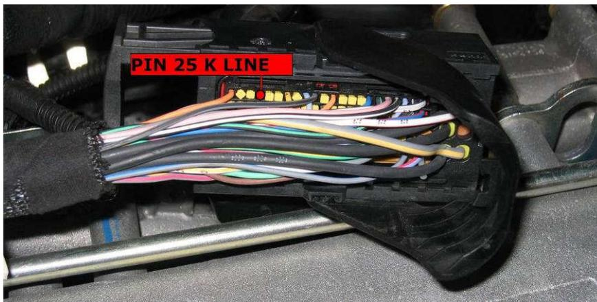
To create the connection we have chosen to connect the K-line (yellow wire of the universal cable) to PIN 43 using the blue wire, after we have connected with the clamps the red wire to the positive pole of the battery (+12V) and the black wire to ground (GND).
