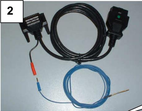
For this wiring you could find an OBDII socket or a typical Mercedes diagnosis connector
