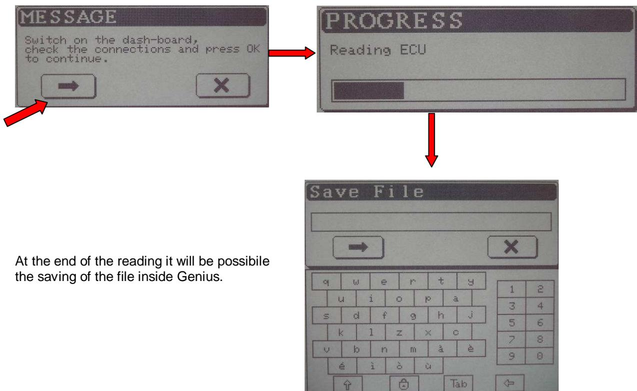
At the end of the reading it will be possibile the saving of the file inside Genius.
