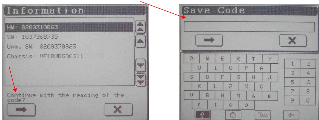
3 – after reading the injectors code it is possibile to read the whole file of ECU, export i tinto Race EVO and manage the modifications.
