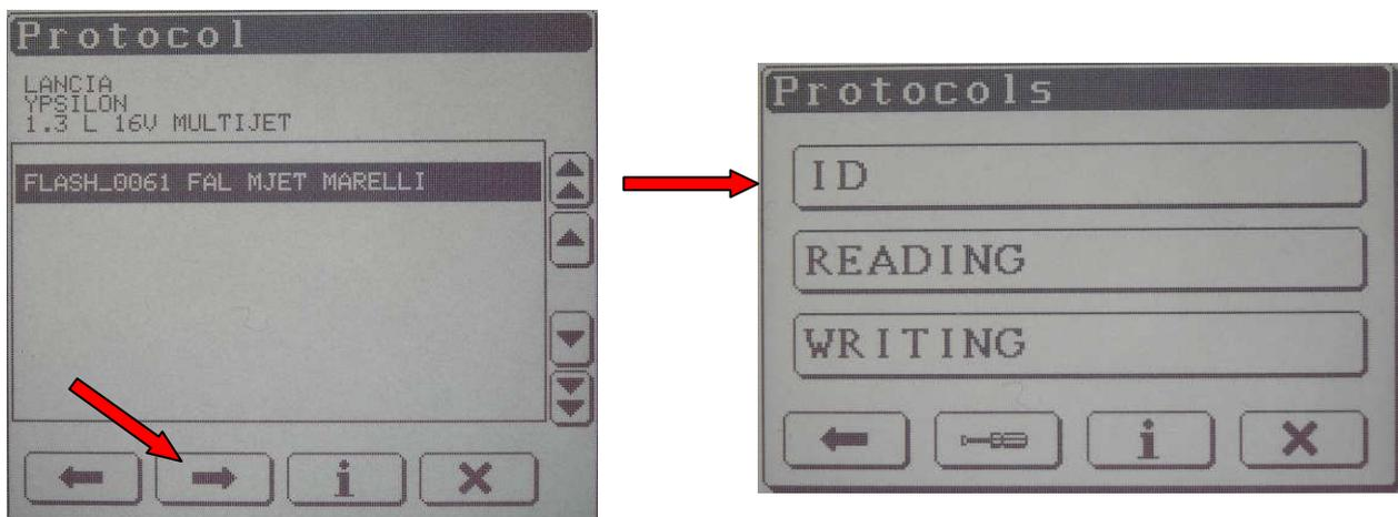
3. After the selection of ID Genius will ask to switch on and off the dash-board and ECU information will be displayed, it is possible to save all the information of the ECU.
