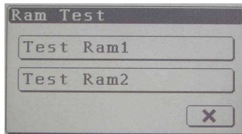
Following the instructions of the Ram test of Genius it is possible to check the execution and final result, after the Test Genius will ask to reset the system.
