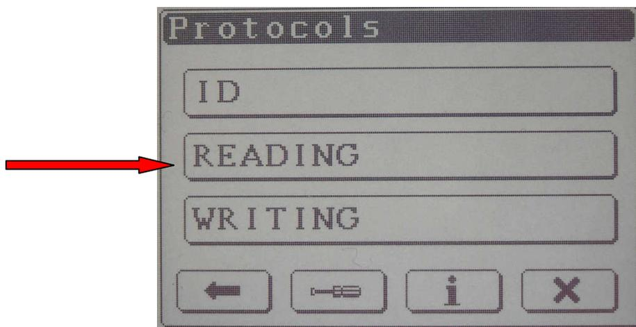
2. After the visualisation of ID Genius will ask to switch on and off the dash-board (this procedure is required to verify the data).The reading progress bar will be displayed. After the reading we will have the file that is inside the ECU of the vehicle.
