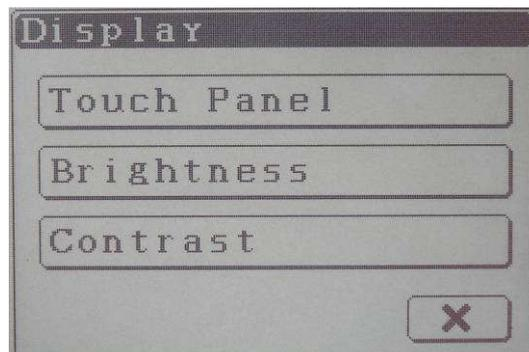
**Touch Panel:** it enables the calibrating of the Touch Panel. The procedure ask to touch with the pen the four corners, suggested by the square, of the Touch Screen.
