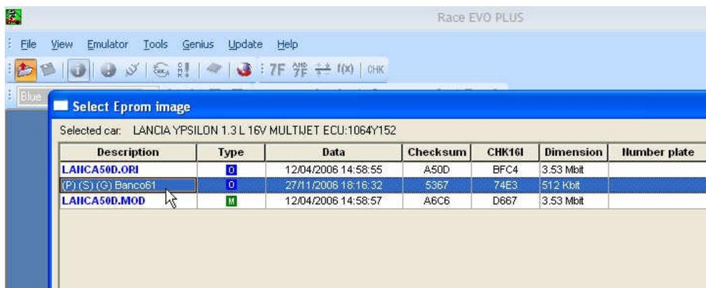
Now it is possible to load the file read from the vehicle and manage the modifications required.
