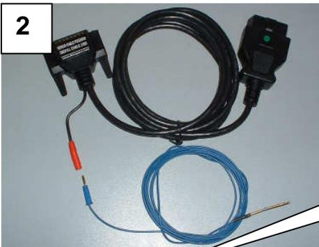
For this kind of connection you could find an OBDII socket or a typical FIAT/ALFA/LANCIA diagnosis connector
