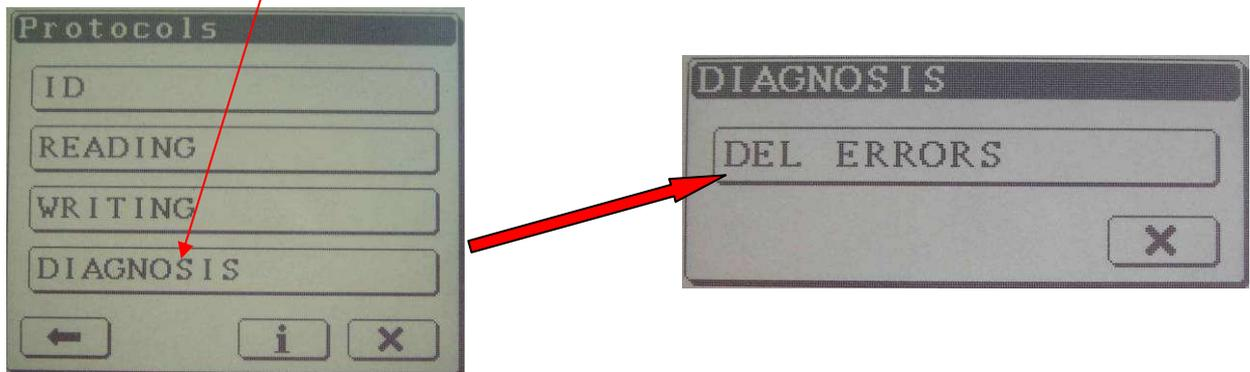
After it will be necessary to follow the procedure required by Genius, switch on the dash-board, a window with the processing bar will open then at the end of the procedure of errors deleting a message will ask to switch off the dash-board.
