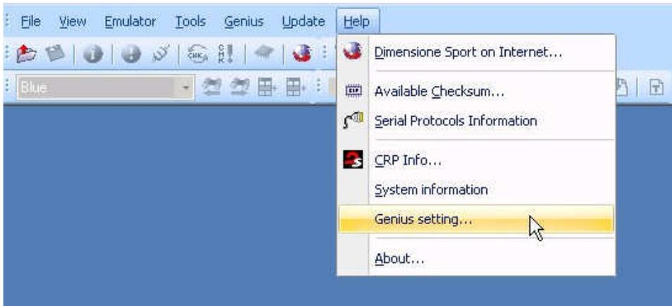
This option allows to check all the features and contracts enabled on Genius. Bottom left there is one of the most important data it is always required by the Technical Support: GOS Version (Genius Operative System).
