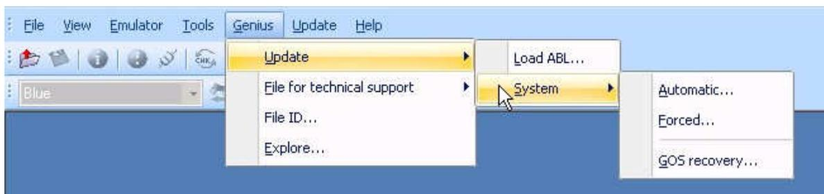
Selecting **Automatic** Race EVO will verify and compare the versions of all the files of the GOS loaded on Genius with the last versions available. If there are some updates available they will be downloaded and automatically installed on Genius.
