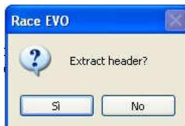
**DON'T EXTRACT:** the file of the vehicle with HEADER will be saved inside the folder. Following this procedure during the writing of the modified file inside ECU the Genius will know that the chosen file is correct for the ECU because the Genius will read the HEADER.
