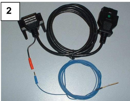
If there is not any communication with the ECU through OBDII socket the only way to communicate is through universal wiring as explained below.
