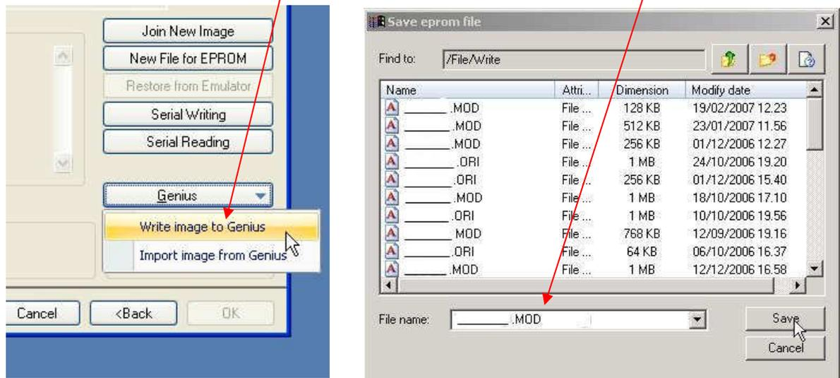
In order to be sure that the selected file has been correctly saved on Genius open the connection through the function Explore, open the folder File and check if inside the folder "Write" there is the file .MOD just imported.
