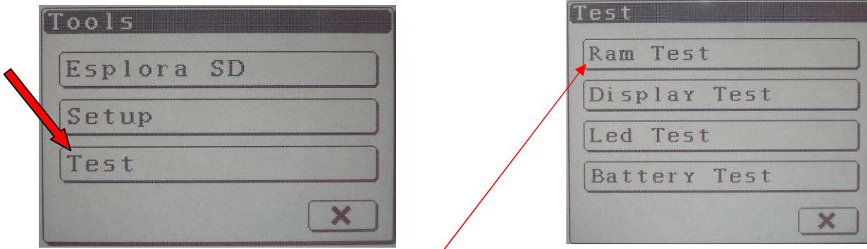
In Tools→Test menu two different kinds of Ram test are available, Ram Test2 is a more detailed and deep analysis to run only after the request of the technical support.
